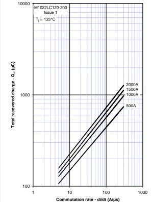
Figure 3 - Recovered charge, Q<sub>rr</sub>
